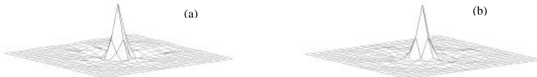
Figure 8: Sampled PSFs after digital filtering. A single digital filter was applied to each of the sampled PSFs of figure 7. The filtered PSF at +20^{\circ}\text{C} is represented by (a), while the filtered PSF at +70^{\circ}\text{C} is represented by (b). The filtered PSF at -20^{\circ}\text{C} is very similar to that of (b). These sampled PSFs are very similar to the sampled PSF of the traditional imaging system of figure 3 at +20^{\circ}\text{C} .
