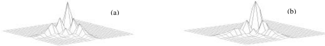
Figure 7: Sampled PSFs of Wavefront Coded system. (a) represents the sampled PSF at +20^{\circ}\text{C} while (b) represents the sampled PSF at +70^{\circ}\text{C} . Sampled PSF at -20^{\circ}\text{C} is similar to that at +70^{\circ}\text{C} . Notice that these sampled PSFs are very different from the sampled PSFs of figure 3 from the traditional imaging system, and by design these sampled PSFs are also very similar to each other by design.
