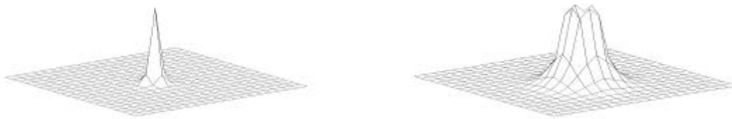
Figure 3: Sampled point spread functions as a function of temperature for the traditional imaging system of figure 1. Sampling is with 20 micron square pixels with 100% fill factor. Left graph represents the sampled PSF of the system at +20°C. The right graph represents the sampled PSF when the temperature is +70°C. The PSF at -20°C is similar to that at +70°C. This system cannot maintain spatial resolution over the temperature range design goal of -20°C to +70°C.
